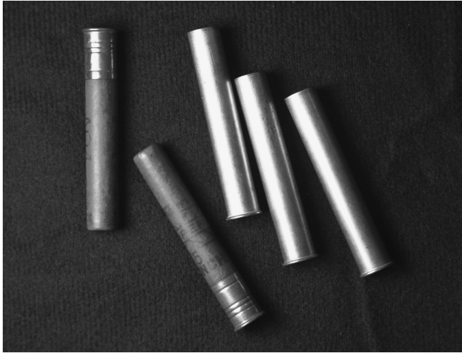
Figure 2.8 Examples of .410 shot shells constructed of brass and paper. The paper shot shells are vintage Winchester Super X; the brass shells were produced by the Russian firm Barnaul. (Images from author's collection.)
